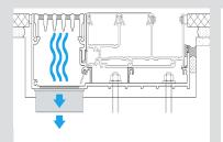
Single-level set down allows outstanding drainage and fast, easy installation.
